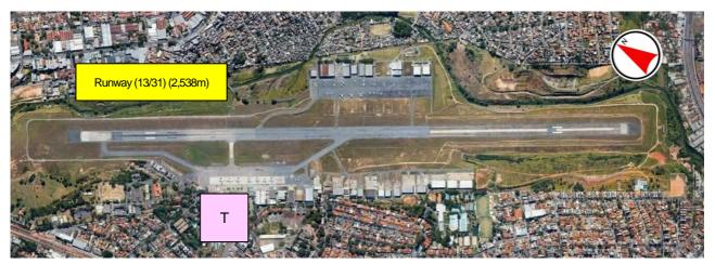
There is a single runway (13/31) with a length of 2,538m. Since 2009, the airport has been equipped with LOC and DME instrument landing systems, which allow the airport to operate under adverse conditions with the same level of operational safety and help reduce the number and time of airport closure by bad weather.
